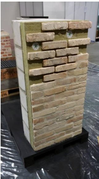
Figure 16. Demolition of external brick work, new thicker insulation and brick tiles- solution does not require additional foundation but might require lintels.
