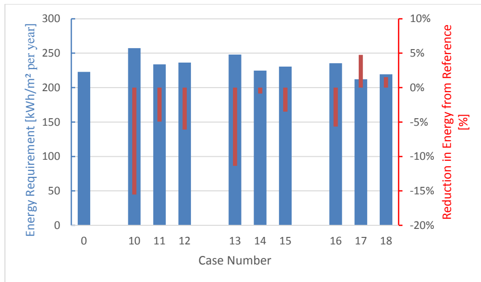
Figure 3. Energy requirement for cases with/without mechanical ventilation at different infiltration levels. Case numbers on the x-axis correspond to Table 3.
