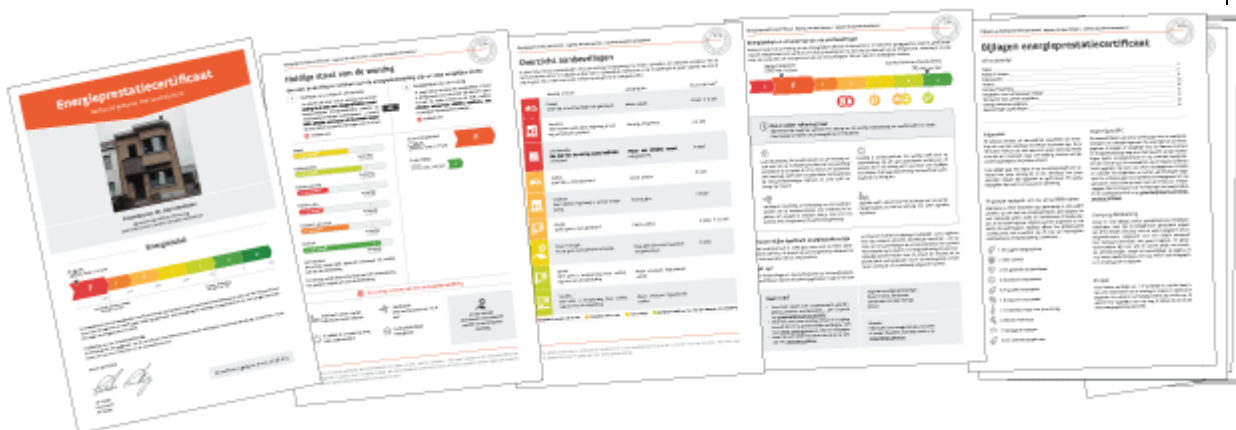
Figure 1: Snapshot of Mijn Energiekompas (above). The choice was made to use energy labels instead of numerical value to represent the energy performance of the dwelling in an intuitive and easily understandable way. The new format of EPCs in Flanders, which will be launched in 2019 (below) will follow the same logic.
