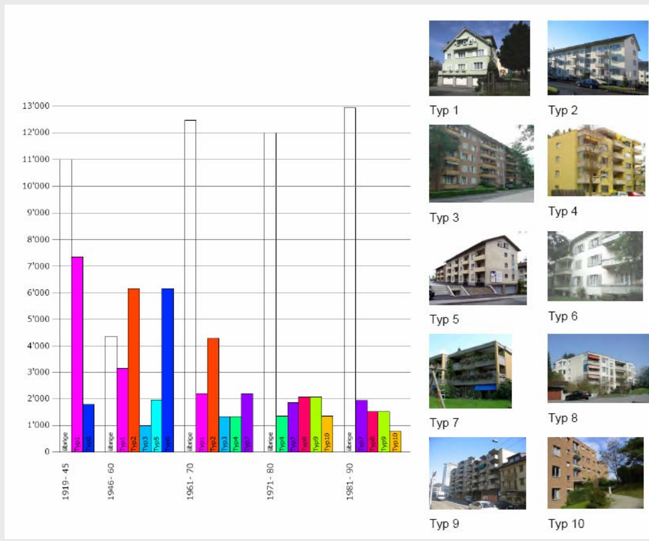
Figure 72: Swiss multi-family house types (diagramme on the left: frequency depending on construction periods) [Fischer 2008] 2
